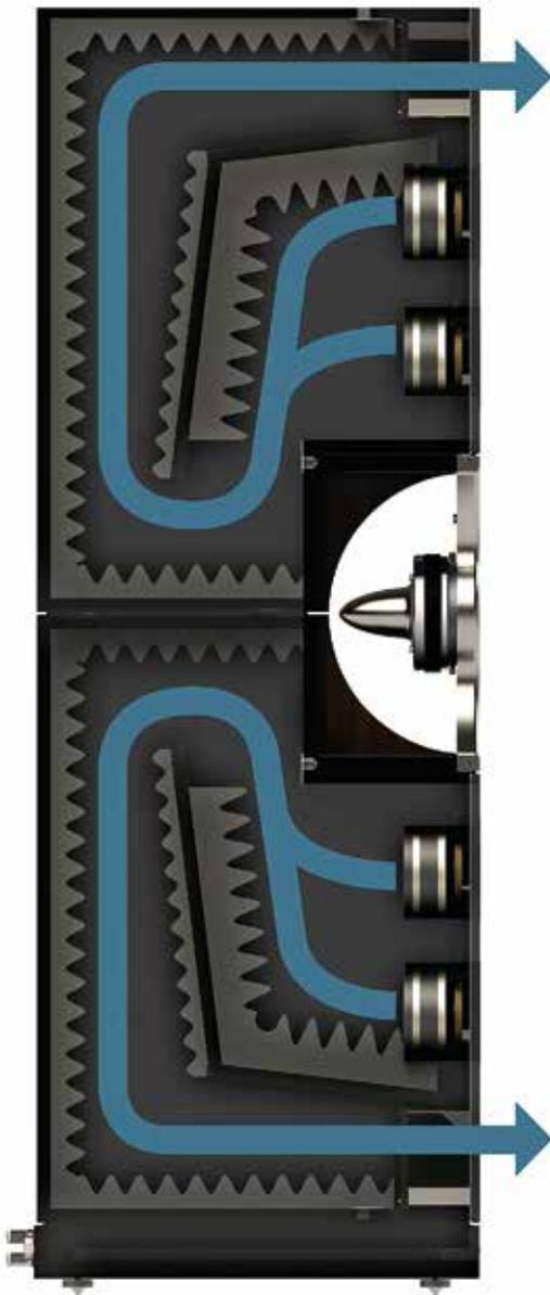
**LEFT:** The fenestria is divided into two mirror-image cabinets where the pairs of 165mm cellular/carbon-fibre bass 'piston drivers' feed into folded 2.4m transmission lines that exit at the very top and bottom of the enclosure
