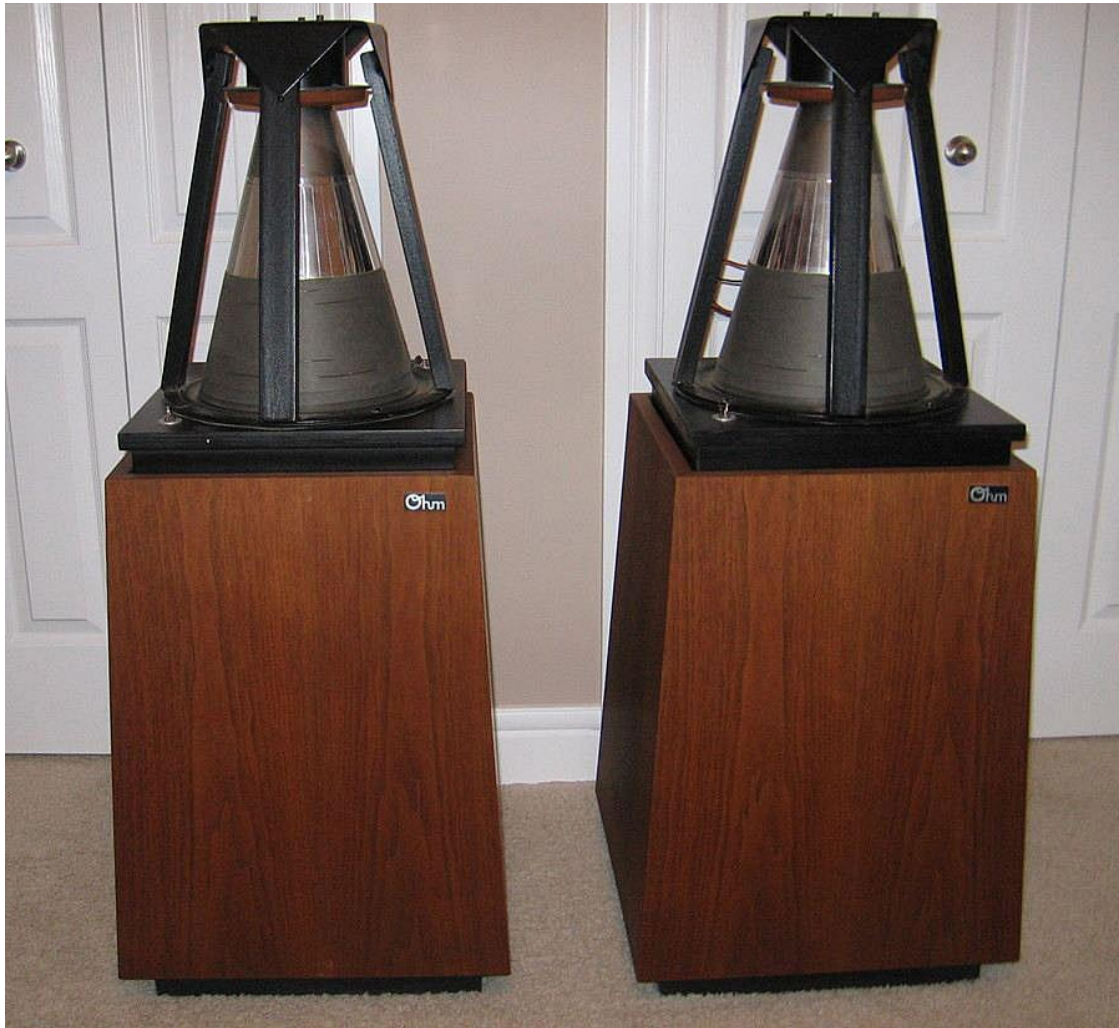
Figure 1. Ohm F loudspeaker with Walsh driver
